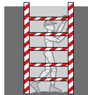
Do not enter an excavation without trench shoring
